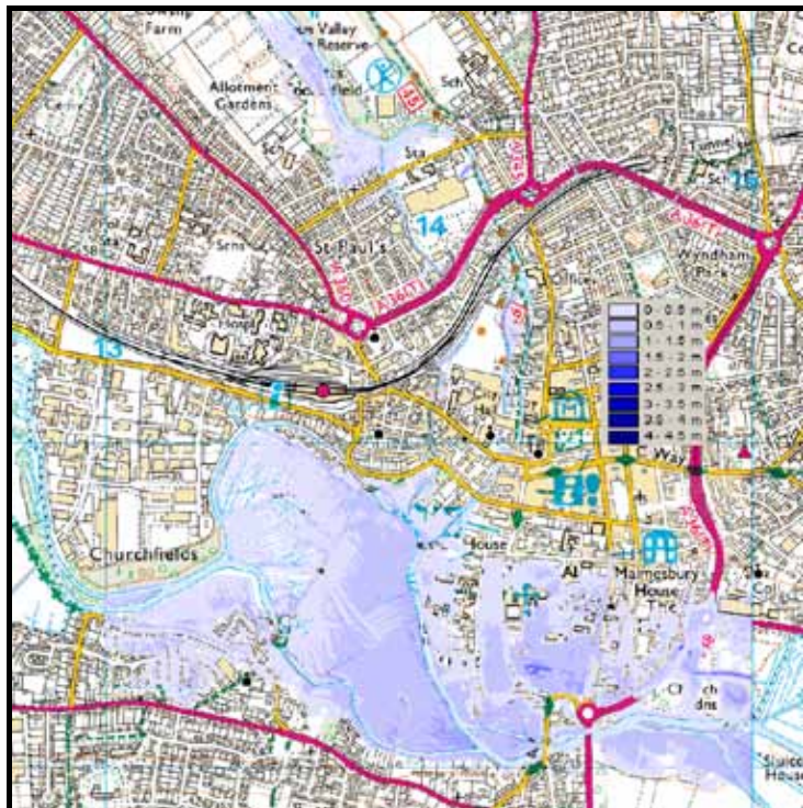
Figure 6.6 Variation in flood depth for the River Avon, Nadder, Bourne and Wylde at Salisbury
